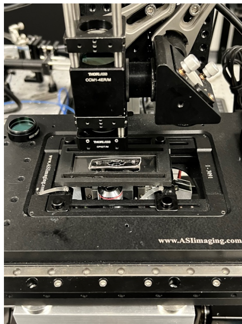
Figure 8 – The microfluidic device is mounted in the microscope with the punched inlet and outlet allowing the sample to be pumped in and through the vasculature-depicting channels. The entire duration of when the liquid was flowing through the device was recorded as a video sequence and subsequently reconstructed for intensity and phase information (Figure 9).
